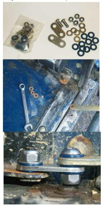
Whereas in this case the vehicle is fitted with floor mats - and it has been necessary to turn the bolt upside down - the head of the bolt is much slimmer than the nut, providing additional clearance.
